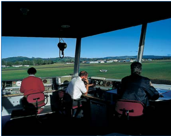
Control towers are the most visible ATC facility, and they are located on, or overlooking, aerodromes. They provide an ATC service within the vicinity of the aerodrome, primarily using visual observation of the aerodrome and circuit.
